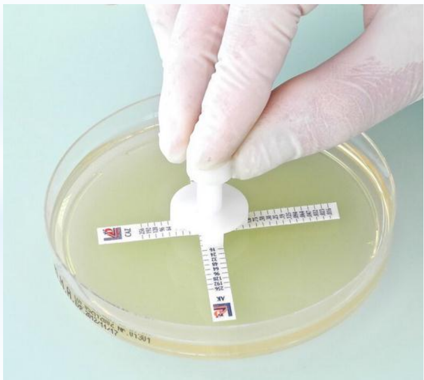
Figure 1, left – MTS Synergy Applicator System™ and MTS Synergy Delivery Tool™ Figure 2, right – MTS Synergy Delivery Tool™: the strips are moved onto the agar surface
